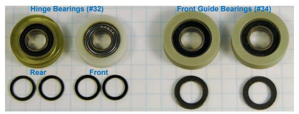
This *Quiet Guide-Bearing Kit* consists of 4 bearings and their associated spacing washers. The kit replaces the steel guide bearings in your 1985-1991 (including some 1984's) Vanagon.
